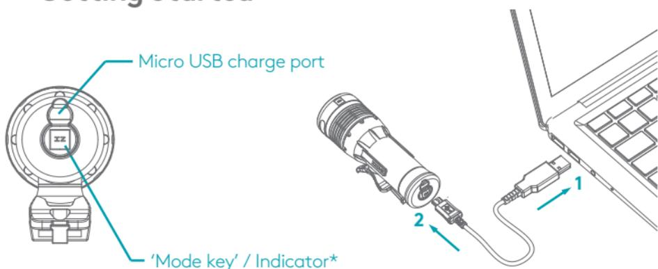
Charge the Arc by gently pulling back micro USB charge port cover, connect and charge using cable supplied. The Arc can also be charged using a mains USB charger at **5V 1.0A MAX**. 'Mode key' indicator will display solid 'green light' once fully charged.
